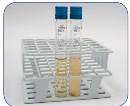
Image 3. After seven days incubation, Bioquell HPV-BIs will provide assurance of a 6-log reduction in bioburden
